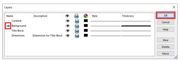
11. Add four layers showed above and double-click the "Background" to set it as a current layer. The "Thickness" of "Background" is set as 0.5mm. Click "OK". We can control the setting of the layers individually like Show/Hide, Colour or Thickness.
