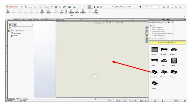
6. Drag and drop an "Isometric" to the drawing area from the "View Palette at "Task Plane". Using other 3D view is also fine.
