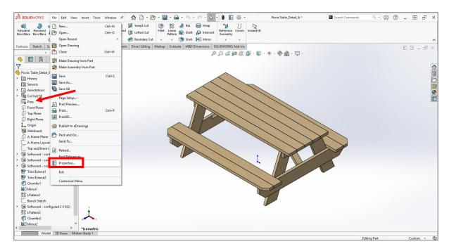
1. Open a part file which has material defined, then open the "Properties".
