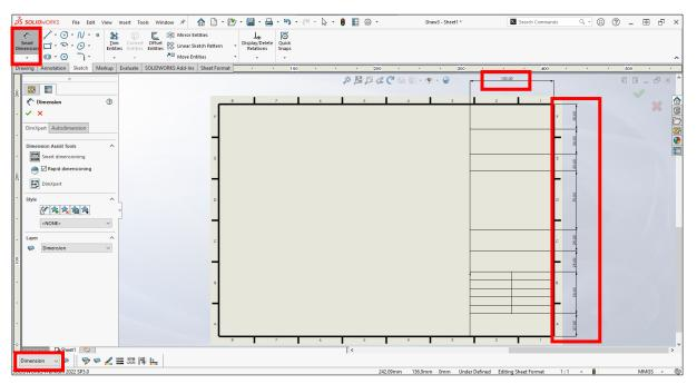
18. Set the "Dimension" as a current layer. Use "Smart Dimension" to define the size of the boxes. It is not necessary to make it be "Fully Defined".
